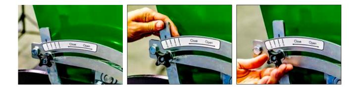
**#4** On the left side of the machine is the Variable Clutch System that controls the rate. To adjust this setting, loosen the 2 knobs on the top of the clutch system box and then rotate the larger knob on the side of the box until you are lined up on the desired number. Tighten the 2 knobs on top to lock in your setting.
