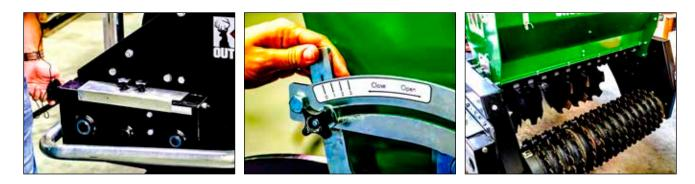
**#1** You will need to find a box or tray that will fit across the width of the seeding elements to catch all of the seed falling from the machine during the calibration process. You will want to mount the box or tray as close to the bottom of the seeding element openings as possible to help you not lose any seed.
