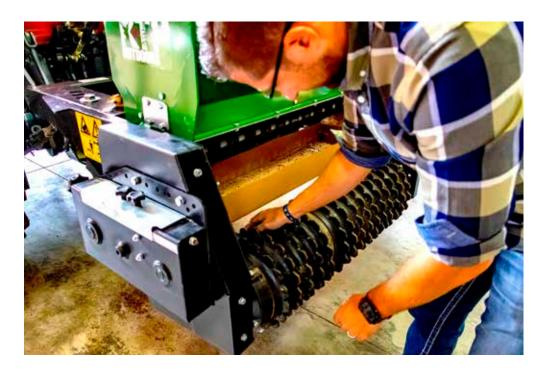
**#7** Carefully remove your seed catching device and empty all of the seed into a box or bucket. We recommend dumping into a larger box first so you don't lose seed on the ground.
