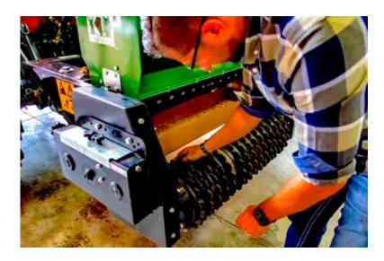
**#2** Open the lid of the seed box and put in your seed of choice. Make sure you fill every seed cup with enough seed for the calibration. If one of the seed cups runs out of seed during this process, the calibration will be inaccurate. Always check the seed cups before and after the calibration.
