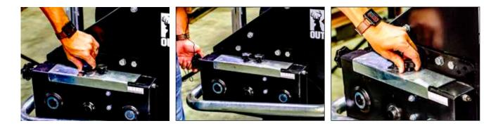
**#5** After verifying that your settings are correct, seed is in all of the seed cups, and the calibration tray is installed properly, use as piece of tape or marking as a set position on the drive wheel.
