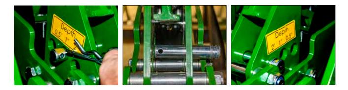
**#13** You will want to adjust the Top Link so that the machine is in a level position. We will use the Top Link to make finer adjustments to the planting depth.
