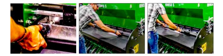
**#2** Open the lid of the seed box and put in your seed of choice. Make sure you fill every seed cup with enough seed for the calibration. If one of the seed boxes runs out of seed during this process, the calibration will be inaccurate. Always check the seed cups before and after the calibration.
