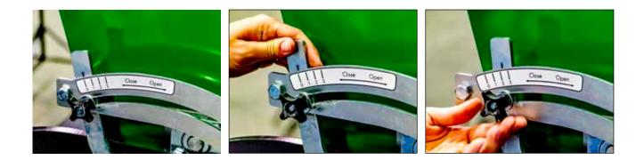
**#4** On the left side of the machine is the Variable Clutch System that controls your rate. To adjust this setting, loosen the 2 knobs on the top of the clutch system box and then rotate the larger knob on the side of the box until you are lined up on the desired number. Tighten the 2 knobs on top to lock in your setting.
