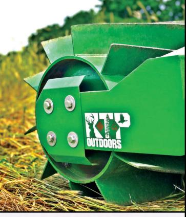
The Goliath Crimper Roller is the perfect tool for wildlife managers wanting to mechanically kill or terminate cover crops without the use of expensive chemicals. Using the Goliath will preserve soil moisture, reduce ground temperatures, prevent weed growth and the terminated cover crop adds a layer of organic, slow release fertilizer at the
